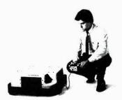
New for 1991 are completely redesigned servo amps, error checking RS-232 communication protocol with selectable 9600/38.4K baud, dual bumper inputs, an enhanced command set, and more.
